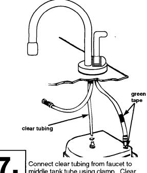
middle tank tube using clamp. Clear tubing may be shortened, if necessary.
